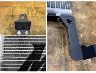
8. Hang the cooler assembly on the hex spacer studs and secure with the included 2X M8 hex nuts. Tighten the nuts hand-tight, allowing for adjustment in further steps. (See image below and on the following page)
