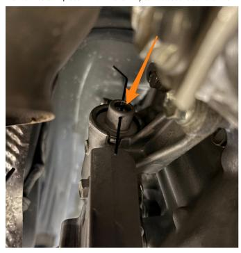
2. Turn the engine on and put the transmission in each gear for about 5 seconds (R, N, D, S) to circulate the transmission fluid now
