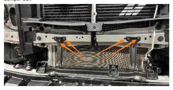
**4.** Remove the 4x push clips and 1x wire harness clip securing the passenger side radiator duct to the core support and other ducting and remove the duct.
