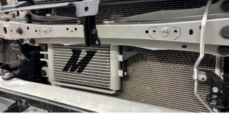
9. Clamp off the lower transmission cooler line that goes into the radiator end tank. Place an absorbent cloth or similar underneath the end of the line to catch any fluid that may spill out when the line is disconnected. Then, remove the clamp from the end of the line and remove the line from the radiator tank.
