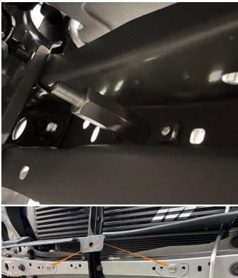
7. Install the 2x included brackets onto the cooler assembly with the included 4x M6 bolts. Tighten the bolts hand-tight, allowing for adjustment in further steps.
