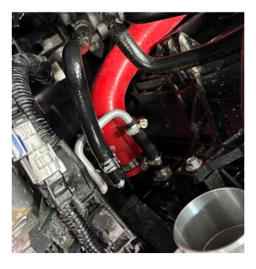
12. Push up on the transmission cooler to move the line assembly away from the plastic duct to the left of the transmission cooler and tighten the 4x 10mm bolts for the transmission cooler bracket and the 2x 13mm nuts securing the transmission cooler to the vehicle. Make sure the lines are clear of any ducting and brackets.
