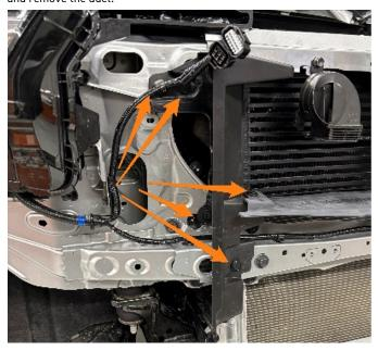
5. Remove the hot side (passenger side) charge air pipe that goes from the turbo outlet to the intercooler. Spread the wire clip on each end and pull away from the turbo and intercooler. (Image on following page)
