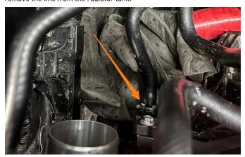
10. Preinstall the included small piece of transmission line onto the line assembly in the location shown. Slide the line on about 25mm/1 inch. Then pre-install 4x included clamps onto the line assembly, in the locations shown. Note the orientation of the clamps but do not tighten yet.
