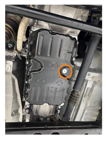
**4.** Coat the seals of the drain and fill plug with ATF and tighten the fill plug to 30ft-lbs and the drain plug to 29 ft-lbs. Remove the 1.5mm allen key (or pin) being used to bypass the transmission thermostat.
