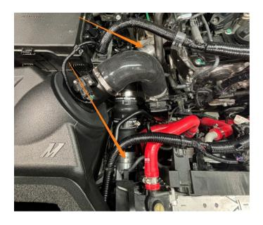
**6.** Install the 2x hex spacers from the transmission cooler kit onto the bumper support bar in the locations shown. Secure with the included M8 13mm bolt. Make sure the spacer and bolt are centered in the hole if possible.
